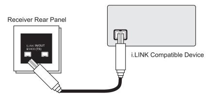
Connect the i.LINK cable from the back of the receiver to the back of the i.LINK compatible device.
